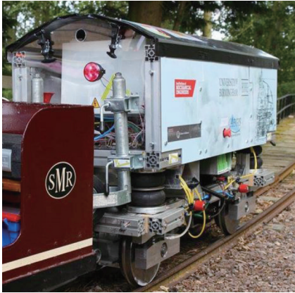
图10 伯明翰大学研制的氢燃料电池动力试验原型机车 Fig.10 Hydrogen fuel cell-powered experimental prototype locomotive developed by the University of Birmingham
